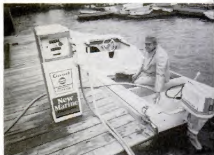
SINCE 22-FOOT HULL PLANED with 45-hp Chrysler engine, gas consumption was far less than it would have been with a larger outboard. With 18-gallon integral tank, we made just two fuel stops on trip
